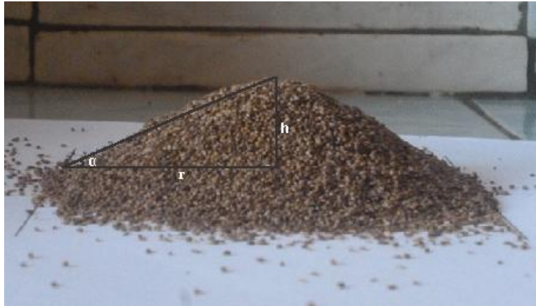
Figure 2: Acha Heap used to Determine Angle of Repose
